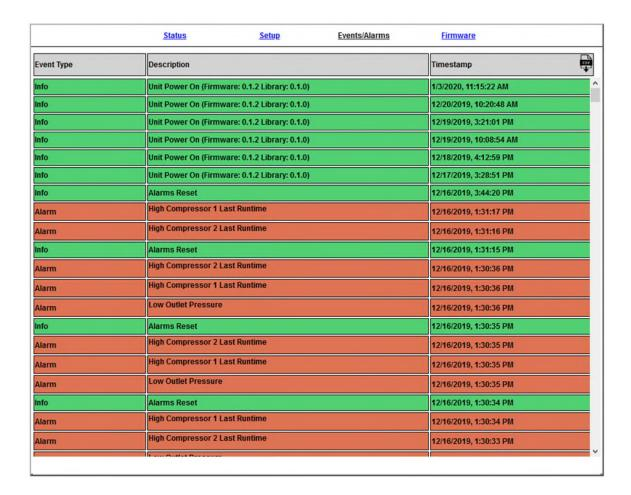
Displays all events such as alarms, changes made, and alarm resets registered by the BD8400W Series Air-dryer. This screen is informational only. You may download a .csv file with all event/alarm information by clicking on the "Download CSV" button at the top right hand corner of the table.
