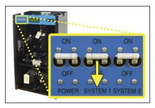
9.13.3 When the System\* Screen(8.4.5.3) appears on the display, press the HOLDButton on the Front Panel to freeze that screen.
