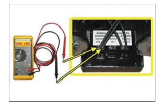
The voltage should measure 106 Volts DC.
