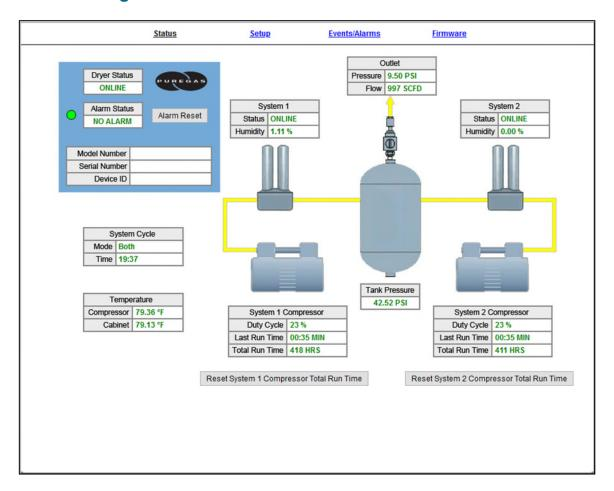
The Status Screen Displays the readings and alarms monitored in the BD8400W Series Air-dryer. Provides remote ALARM RESET.
