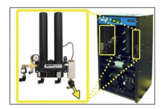
6.5.16.2 Turn the knob until the reading on the pressure gauge is 50PSI.
