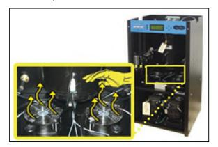
If either fan is not blowing air upwards as described:
