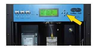
**9.15.3** Make a note of the current Outlet Pressure (**OUTP**) reading.
