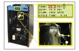
If the Compressor Cycling fails either test described, it indicates a problem with the Control Board which may need to be replaced. See sections 11.1 for part detail and 11.7 for ordering information.
