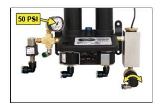
**6.5.17** Let the dryer run until the Humidity drops under 2% on both System 1 and System 2 (may take up to 15 minutes).
