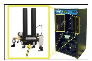
**9.8.3** Use a Voltmeter to measure the DC voltage across each set of "106VDC" terminals.
