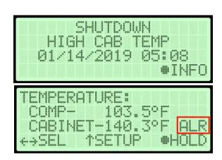
**SHUTDOWN** mode to protect against damage due to overheating.
