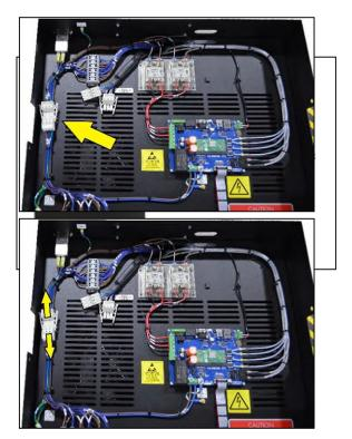
**6.5.13.2** Locate the Main Power Lead quick disconnects in the top section of the dryer.
