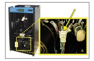
9.3.3 Use a Voltmeter to measure the voltage between the Hot and Neutral wires by placing the probes in the openings in the power connector:
